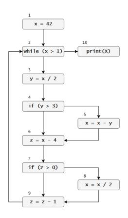
First we should make the CFG (Control Flow Graph) that models the program behaviour.
